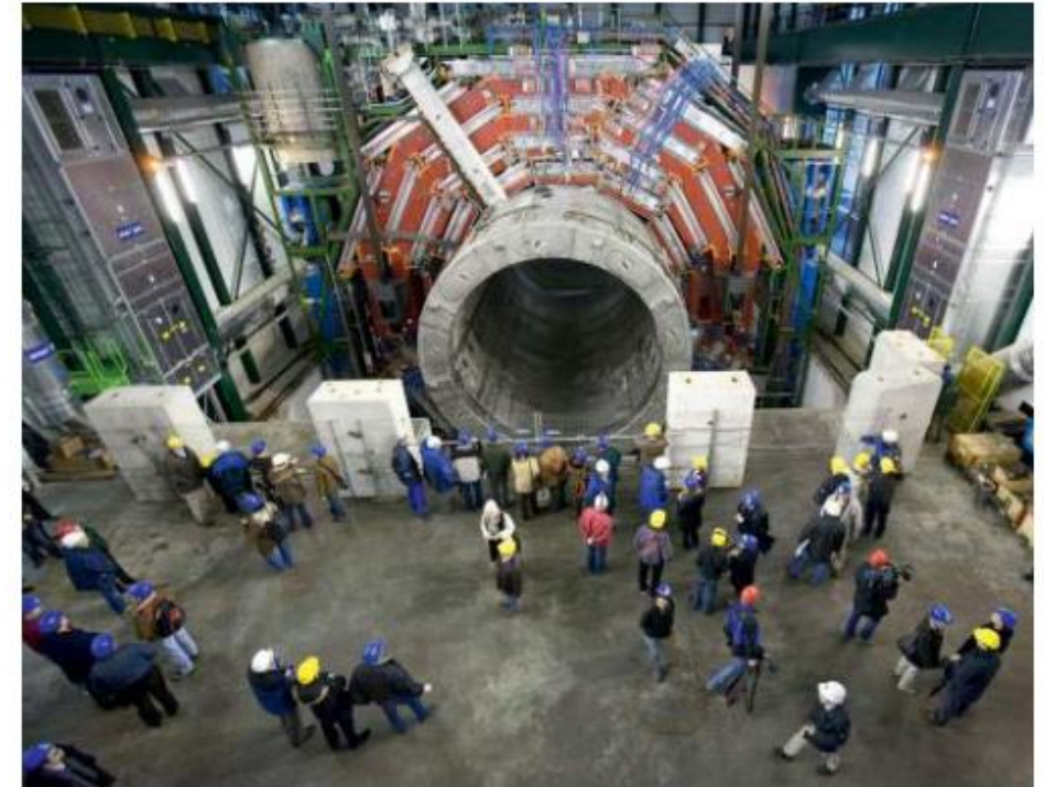
Figure 16.10 Particle accelerators have become bigger and bigger as scientists have sought to look further and further into the fundamental nature of matter. This is one of the particle detectors of the Large Hadron Collider (LHC), as it was about to be installed. The entire collider is 27 km in circumference.
